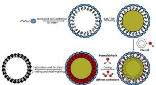
Fig. 1 Synthesis procedure of a sulfur-particle-templated resole resin
