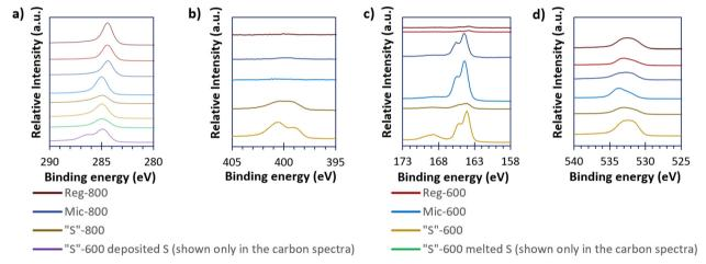
The high resolution XPS spectra of the carbonaceous (and the "S"-600/S composites) materials of C 1s (a), N 1s (b), S 2p (c), and O 1s (d)
