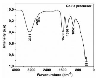
Fig. 1 FTIR of the Co-Fe precursor
