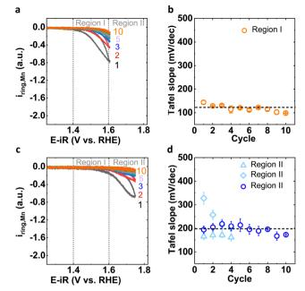
Fig. 2 (a) Mn corrosion current observed at Pt ring for 1st to 10th cycle before OER (in potential window of 1.25-1.6 V vs. RHE) and (b) corresponding Tafel slope in Region I. (c) Mn corrosion current observed at Pt ring for 1st to 10th cycle after the conditioning process (in potential window of 1.25-1.75 V vs. RHE) and (d) corresponding Tafel slopes in Region II. Cycles are indicated by coloured numbers.
