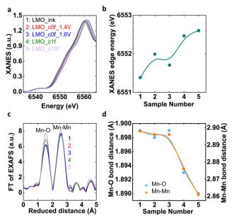
Fig. 4 (a) XANES spectra at Mn-K edge and (b) corresponding relation of XANES edge energy with LMO\_ink and electrochemically processed samples. (c) FT of EXAFS spectra at the Mn-K edge and (d) corresponding relation of Mn-O and Mn-O bond distances with LMO\_ink and electrochemically processed samples. Lines are guide to the eye in panels b and d. Coloured numbers refer to sample numbers from the legend in panel a and Table 1.
