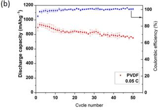
Fig. 3 (a) Variation of discharge capacity for 2 cells with polar PVDF separator in differing orientations of the film relative to the anode. (b) Variations (expressed as mean and standard deviation) of discharge capacities for 3 cells of each type and with polar PVDF separator in the H-side configuration. All measurements were made at 0.05C.
