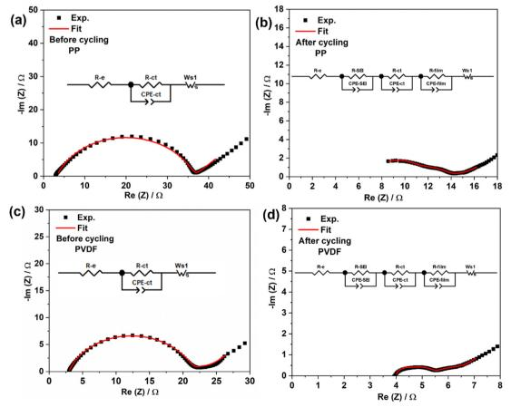
Fig. 5 Nyquist plots for LSB cells before and after cycling with (a), (b) PP and (c), (d) PVDF separators. The equivalent circuit parameters: R-e = electrolyte resistance, R-ct = charge-transfer resistance, R-SEI = resistance of solid electrolyte interphase, R-film related to Li<sub>2</sub>S/Li<sub>2</sub>S<sub>2</sub> film, and Ws. CPE-ct, CPE-sd, CPE-SEI and CPE-film represent constant phase elements associated with R-ct, R-SEI and R-film respectively
