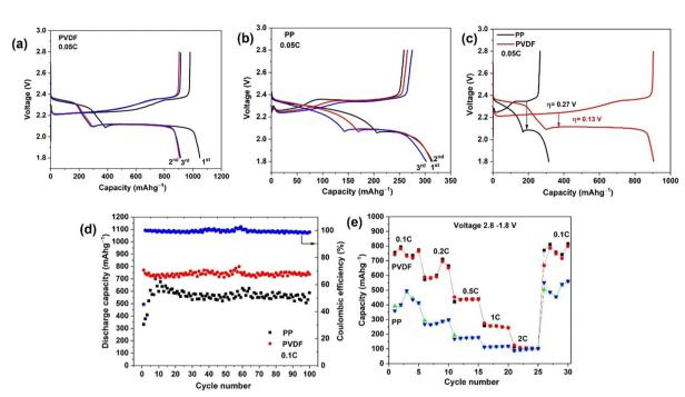
Fig. 4 Initial discharge/charge voltage profiles of a Li-S battery at current rates of 0.05C using (a) PVDF and (b) PP separator. Also (c) galvanostatic discharging/charging performance of Li-S batteries with different separators at 0.05C and (d) cycling performance of the Li-S batteries with different separators at 0.1C, (e) rate capability performance of Li-S batteries with different separators at various current rates ranging from 0.1 to 2C, and returning to 0.1C
