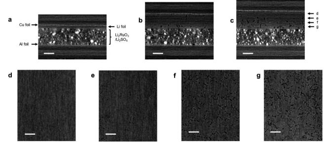
Fig. 6 (a)-(c) X-ray CT images of cell B; (a) as prepared, (b) after the 10th cycle, and (c) after the 20th cycle in the cross-sectional direction; (d)-(g) X-ray CT images of cell B after the 20th cycle in the surface direction. Scale bars are 100  $\mu m$ .
