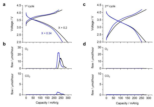
Fig. 4 (a) and (c) Charge/discharge profile for 1st and 2nd cycle; (b) and (d) generated gas profile in the (b)1st and (d) 2nd cycles in an electrochemical cell equipped with  $\text{Li}_2\text{RuO}_3/\text{Li}_2\text{SO}_4$  samples (black curve: x=0.2 and blue curve: x=0.34) as positive electrodes.
