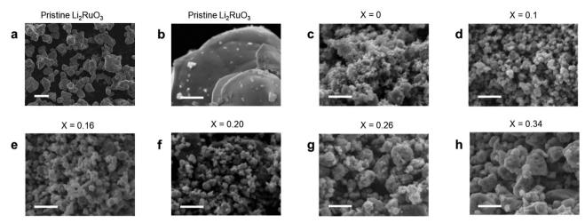
Fig. 2 SEM-EDS images of (a) and (b) pristine Li<sub>2</sub>RuO<sub>3</sub> and (c)-(h) Li<sub>2</sub>RuO<sub>3</sub>/Li<sub>2</sub>SO<sub>4</sub> samples. Scale bars are (a) 10 μm and (b)-(h) 1 μm.
