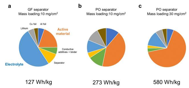
Fig. 1 Weight fractions of LMB components calculated using the parameters listed in Table S1 (ESI†). (a) Glass fiber separator, a mass loading of 10 mg cm<sup>-2</sup>, (b) polyolefin separator, a mass loading of 10 mg cm<sup>-2</sup>, and (c) polyolefin separator, a mass loading of 30 mg cm<sup>-2</sup>.
