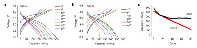
Fig. 5 (a) and (b) Charge/discharge profile of the electrochemical cell equipped with the  $\text{Li}_2\text{RuO}_3/\text{Li}_2\text{SO}_4$  sample (x=0.2) as the positive electrode: (a) cell A and (b) cell B. (c) Discharge capacity plotted against the cycle number for cell A (black curve) and cell B (red curve).
