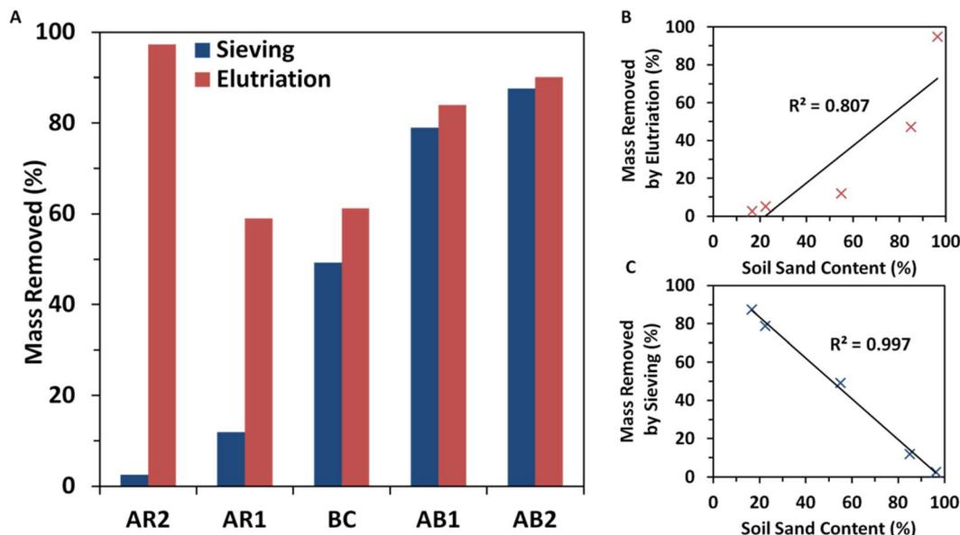
Fig. 1 Total sample mass removal by pretreatment for each sample and method (A), and sample mass removal solely by elutriation (B) and sieving (C) as a function of soil sand content. Arkansas River 2 (AR2), Arkansas River 1 (AR1), Boomer Creek (BC), Applied Biosolids 1 (AB1), and Applied Biosolids 2 (AB2).
