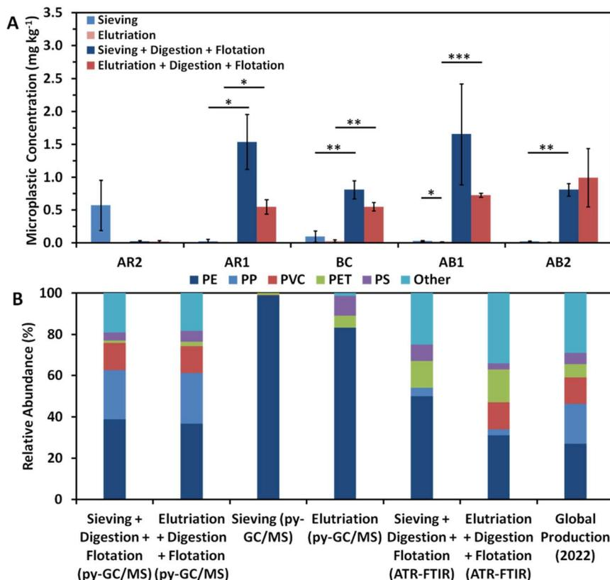
Fig. 3 Soil microplastic concentration ( $\text{mg kg}^{-1}$ ) measured by py-GC/MS for all methods (A). Relative abundance for all methods in terms of concentration (py-GC/MS) and number of identified polymers (ATR-FTIR) compared to 2022 global polymer production (B). \* denotes  $p < 0.05$ , \*\* denotes  $p < 0.01$ , \*\*\* denotes  $p < 0.005$ . Error bars denote standard error.
