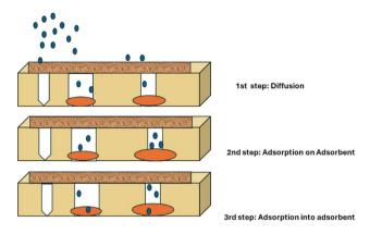
Fig. 3 Mechanism of classical adsorption.
