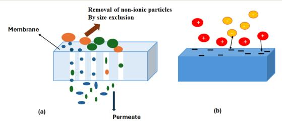
Fig. 4 (a) Removal of non-ionic particles by size exclusion and (b) Donnan exclusion; attraction of positive ions by a negatively charged membrane.
