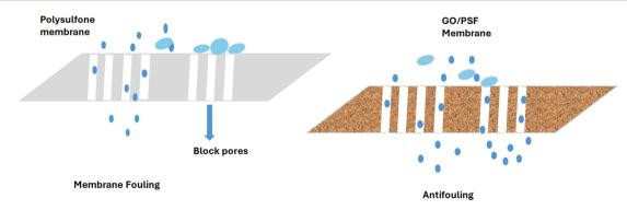
Fig. 5 Fouling and antifouling behaviour of PSF and GO/PSF.
