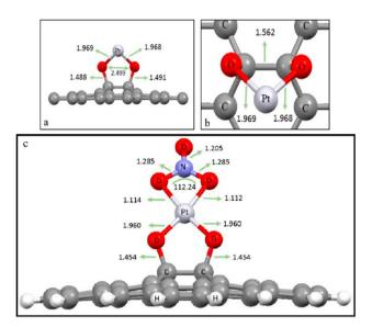
(a and b) Side view and top view of the optimized position of Ptnanoparticles on the surface of GO, and (c) optimized nitrate-interaction with the GO/Pt surface and bond lengths (Å).199
