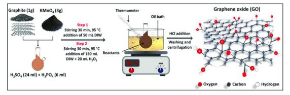
Fig. 1 GO synthesis by a modified Hummer's method. 57
