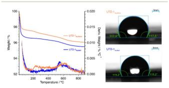
Fig. 2 (Left) Thermal gravimetric profiles for detemplated UTD-1 variants. Data gathered under air atmosphere. (Right) Water contact angle measurements for UTD-variants.
