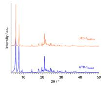
Fig. 1 Powder X-ray diffraction patterns for detemplated UTD-1 (DON) variants.
