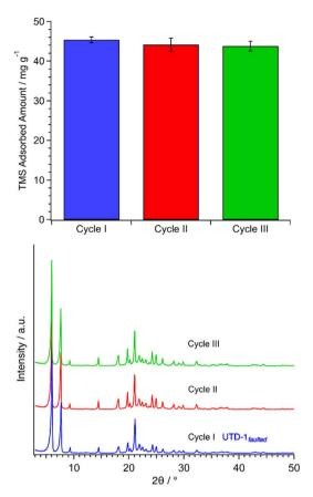
Fig. 7 (Top) Adsorbed amount of TMS onto fresh and regenerated UTD-1<sub>faulted</sub>. (Bottom) XRD pattern of UTD-1<sub>faulted</sub> prior to each adsorption cycle. The initial TMS concentration during the adsorption tests was 125 mg  $L^{-1}$ . Adsorbent regeneration was performed through thermal treatment and rehydroxylation.
