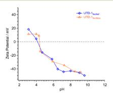
Fig. 3 Zeta potential measurements for UTD-1 materials.
