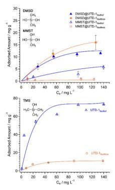
Fig. 4 Single component equilibrium adsorption isotherms for (top) MMST and DMSD, and (bottom) TMS onto UTD-1. Conditions: ambient temperature and pH  $\sim$  7. Data includes error bars.
