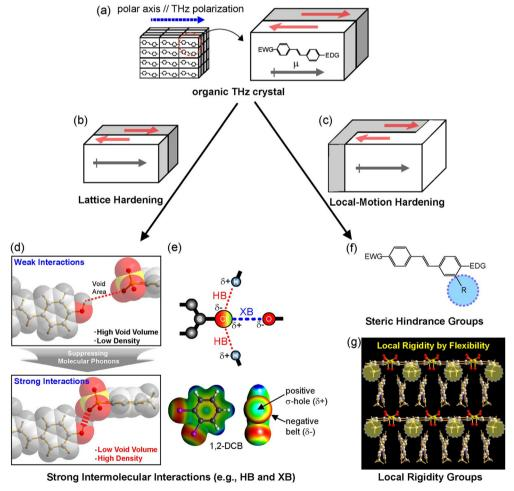
Fig. 6 Schematics of strategies for suppressing phonon vibrations of (a) benchmark organic THz crystals: (b) lattice hardening by (d) and (e) introducing strong intermolecular interaction groups and (c) local-motion hardening by (f) introducing steric hindrance group and (g) local rigidity group with a high conformational freedom. Reproduced and adapted with permission. 55,73,76,77 Copyright 2022 and 2023, Wiley-VCH.
