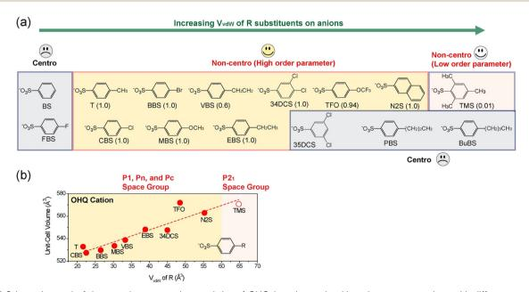
Fig. 5 (a) Schematic trend of the crystal structure characteristics of OHQ-based crystals with various counter anions with different van der Waals volume,  $V_{\text{vdW}}$  of R substituents. (b) The corresponding volume of a cation-anion pair (unit-cell volume divided by the crystallographic Z number) as a function of van der Waals volume, V<sub>vdW</sub> of R substituents. Reproduced and adapted with permission.<sup>74</sup> Copyright 2023, Wiley-VCH.
