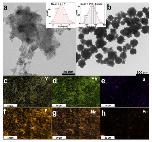
Fig. 2 The representative TEM images of the FeS<sub>2</sub> NPs (a) and FeS<sub>2</sub>@NaYF<sub>4</sub>:Yb<sup>3+</sup>,Er<sup>3+</sup> NC (b); the insets show histograms of the NPs and NC size distribution. The EDX mapping of elements in the FeS2@NaYF4:Yb3+,Er3+ NC, i.e., Y (c), Yb (d), S (e), F (f), Na (g), Fe (h).
