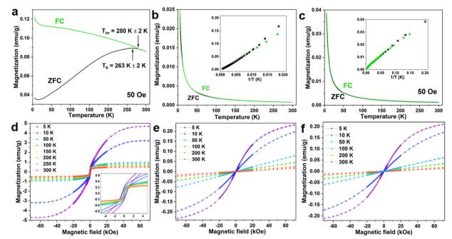
Fig. 6 ZFC-FC curves of the FeS<sub>2</sub> core (a), the NaYF<sub>4</sub>:Yb<sup>3+</sup>,Er<sup>3+</sup> NPs (b) and FeS<sub>2</sub>@NaYF<sub>4</sub>:Yb<sup>3+</sup>,Er<sup>3+</sup> NC (c). Magnetic-field dependence of magnetization at temperatures: 5 K, 10 K, 50 K, 100 K, 200 K, 250 K, and 300 K for the FeS<sub>2</sub> core (d), the NaYF<sub>4</sub>:Yb<sup>3+</sup>,Er<sup>3+</sup> NPs (e) and FeS<sub>2</sub>@NaYF<sub>4</sub>:Yb<sup>3+</sup>,Er<sup>3+</sup> NC materials (f).
