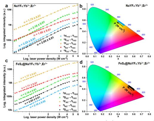
Fig. 4 Integrated luminescence intensity as a function of laser power density for the NaYF<sub>4</sub>:Yb<sup>3+</sup>,Er<sup>3+</sup> NPs (a) and FeS<sub>2</sub>@NaYF<sub>4</sub>:Yb<sup>3+</sup>,Er<sup>3+</sup> NC (c). CIE diagrams for the NPs (b) and NC (d) showing the color coordinates as a function of laser power density.
