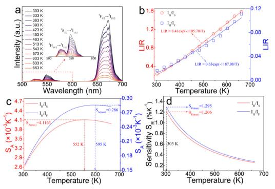
Fig. 8 (a) Temperature-dependent UCL emission spectra of the  $(Gd_{0.8}Er_{0.1}Yb_{0.1})(La_{0.9}Sc_{0.1})O_3$  phosphor at 303–663 K under 980 nm laser excitation. The inset shows an enlarged wavelength region from 500 to 600 nm. (b) Relationship between LIR values and temperature. (c) Absolute sensitivity (SA). (d) Relative sensitivity  $(S_R)$
