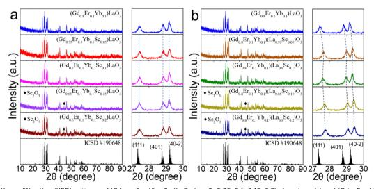
Fig. 1 Powder X-ray diffraction (XRD) patterns of  $(Gd_{0.8-x}Er_{0.1}Yb_{0.1}Sc_x)LaO_3$  (x = 0, 0.05, 0.1, 0.15, 0.2) phosphors (a) and  $(Gd_{0.8}Er_{0.1}Yb_{0.1})(La_{1-x}Sc_x)O_3$ (x = 0, 0.05, 0.1, 0.15, 0.2) phosphors (b). The standard pattern of GdLaO<sub>3</sub> (ICSD#190648) is presented as a reference. The right patterns in pictures (a) and (b) depict an enlarged angular region from 27° to 30°, respectively.
