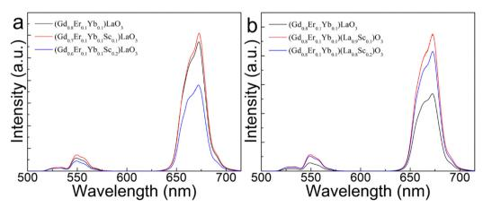
Fig. 4 UCL spectra of  $(Gd_{0.8-x}Er_{0.1}Yb_{0.1}Sc_x)LaO_3$  (x = 0, 0.1, 0.2) (a) and  $(Gd_{0.8}Er_{0.1}Yb_{0.1})(La_{1-x}Sc_x)O_3$  (x = 0, 0.1, 0.2) (b) under 980 nm laser excitation.
