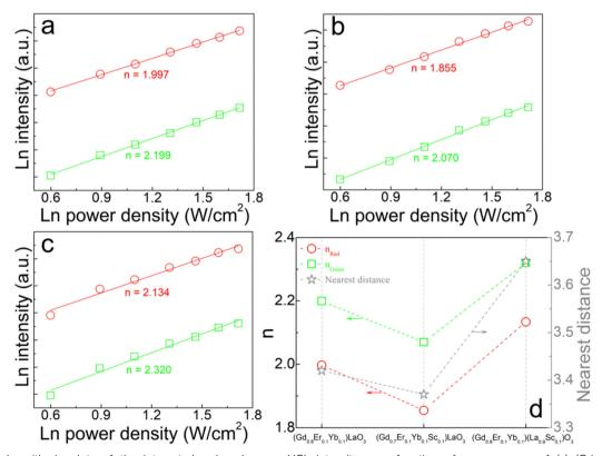
Fig. 6 Double logarithmic plots of the integrated red and green UCL intensity as a function of pump power of (a) (Gd<sub>0.8</sub>Er<sub>0.1</sub>Yb<sub>0.1</sub>)LaO<sub>3</sub>, (b)  $(Gd_{0.8}Er_{0.1}Yb_{0.1}Sc_{0.1})LaO_3$ , and (c)  $(Gd_{0.8}Er_{0.1}Yb_{0.1})(La_{0.9}Sc_{0.1})O_3$ . (d) Relationship between the slope of the curve and nearest distance between Yb<sup>3+</sup> and Er<sup>3+</sup> or Er<sup>3+</sup> and Er<sup>3+</sup> in the host.
