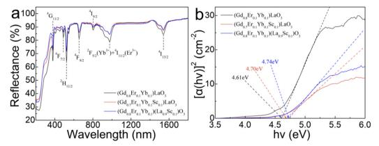
Fig. 2 (a) Diffuse reflectance spectra of  $(Gd_{0.8}Er_{0.1}Yb_{0.1})LaO_3$ ,  $(Gd_{0.8}Er_{0.1}Yb_{0.1}Sc_{0.1})LaO_3$ , and  $(Gd_{0.8}Er_{0.1}Yb_{0.1})(La_{0.9}Sc_{0.1})O_3$  phosphors. (b) Corresponding calculated bandgap values
