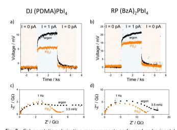
Fig. 2 Galvanostatic polarization measurements performed on horizontal devices with (a) (PDMA)PbI<sub>4</sub> and (b) (BzA)<sub>2</sub>PbI<sub>4</sub> thin films in an argon atmosphere and under iodine atmosphere ( $P(l_2) = 7 \times 10^{-7}$  bar; argon carrier gas) at 60 °C in the dark. Impedance spectra collected under analogous conditions are shown in (c) for the DJ and (d) for the RP film.
