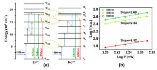
Fig. 12 (a) Energy level transition of Er<sup>3+</sup>-Ho<sup>3+</sup> ions co-doped under 1550 nm excitation. (b) IP curve of Er<sup>3+</sup>-Ho<sup>3+</sup> ions co-doped under 1550 nm excitation.
