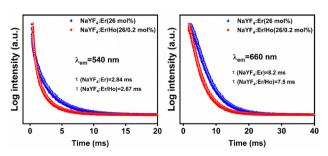
Fig. 14 Fluorescence lifetime of the sample when excited in the 980 nm band.
