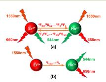
Fig. 13 (a) Schematic diagram of the reverse energy transfer of Er<sup>3+</sup>- $\mathrm{Ho}^{3+}$  ions. (b) Schematic diagram of the energy transfer of  $\mathrm{Er}^{3+}\mathrm{-Ho}^{3+}$  ions.
