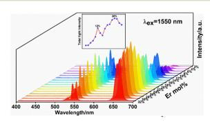
Fig. 5 Upconversion emission spectra from the  ${\rm Er}^{3+}$ -doped samples under 1550 nm excitation.
