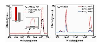
Fig. 10 (a) Upconversion emission spectra of the single-doped sample with  ${\rm Ho^{3+}}$  ions and co-doped sample with  ${\rm Ho^{3+}}$ -Yb<sup>3+</sup> under 1550 nm excitation. (b) Absorption spectra of the samples singly doped with  ${\rm Ho^{3+}}$  ions and singly doped with  ${\rm Er^{3+}}$  ions.
