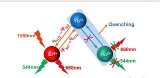
Fig. 17 Schematic diagram of reverse energy transfer of Er<sup>3+</sup>–Yb<sup>3+</sup> ions.
