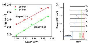
Fig. 11 (a) IP curves of singly doped samples with Ho3+ ions under 1550 nm excitation. (b) Upconversion energy level transition diagram of Ho<sup>3+</sup> ions under 1550 nm excitation
