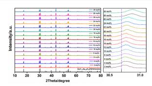
Fig. 1 XRD patterns of doping with different concentrations of Er<sup>3+</sup> ions.
