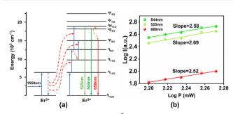
Fig. 8 (a) Energy level transition of Er<sup>3+</sup> ions under 1550 nm excitation; (b) IP curve of Er<sup>3+</sup> ions under 1550 nm excitation.
