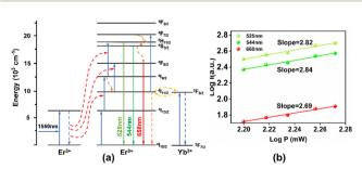
Fig. 16 (a) Energy level transition of Er<sup>3+</sup>-Ho<sup>3+</sup>-Yb<sup>3+</sup>ion triple-doping under 1550 nm excitation. (b) IP curve of Er3+-Ho3+-Yb3+ion tripledoping under 1550 nm excitation.
