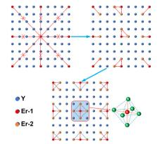
Fig. 7 Schematic diagram of Er<sup>3+</sup> ion doping energy transfer.
