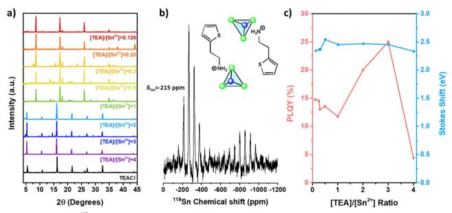
Fig. 4 (a) XRD patterns, (b) 119Sn MAS-NMR spectra measured at room temperature (Inset: probable crystalline structure) and (c) variation of the PLQY and Stokes shift of 0D-[TEASnCl3][TEACl] microcrystals as a function of the molar ratio [TEA]/[Sn<sup>2+</sup>].
