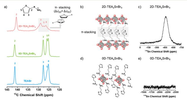
Fig. 3 (a) 13C MAS-NMR spectra of TEABr, 0D-TEA<sub>4</sub>SnBr<sub>6</sub>, and 2D-TEA<sub>2</sub>SnBr<sub>4</sub> powders. Crystalline structures and 119Sn NMR of (b) and (c) 2D-TEA<sub>2</sub>SnBr<sub>4</sub> and (d) and (e) OD-TEA<sub>4</sub>SnBr<sub>6</sub>.
