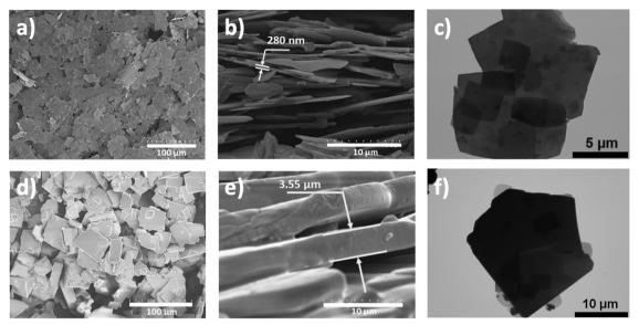
Fig. 1 Top-view SEM (a) and (d), cross-sectional SEM (b) and (e) and TEM images (c) and (f) of 2D-TEA<sub>2</sub>SnBr<sub>4</sub> (a)-(c) and 0D-TEA<sub>4</sub>SnBr<sub>6</sub> (d)-(f) microcrystals.
