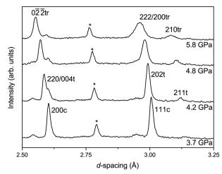
Fig. 6 Changes in diffraction pattern of  $CsCaCl_3$  with increasing pressure across the phase transition region. In the bottom trace the reflections from the cubic (c) phase are identified and those from lead identified by an asterisk. Upon increasing pressure the R point reflection from the tetragonal (t) phase appears (211t) and other reflections are split. At higher pressure the splitting which occurs from the rhombohedral (tr) phase is observed.
