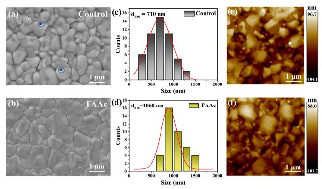
Fig. 2 Top-view SEM images of (a) control and (b) FAAc modified-perovskite films. The grain size distribution of (c) control and (d) FAAc modifiedperovskite films. AFM images of (e) control and (f) FAAc modified-perovskite films.
