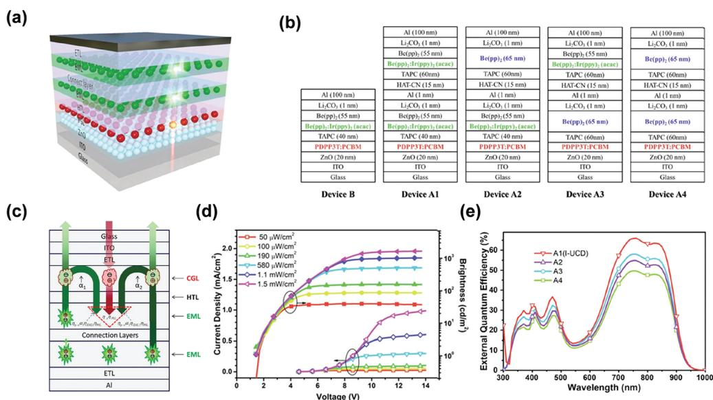
Fig. 8 (a) Schematic diagram of the PD with a Tandem OLED up-conversion device. (b) Structures of different up-conversion devices. (c) Schematic diagram of physical processes involved in the device. (d)  $J$ - $V$  &  $B$ - $V$  characteristics of integrated up-conversion devices under different NIR light powers. (e) EQE spectra of different devices at 9 V bias.<sup>81</sup> Copyright 2018, Royal Society of Chemistry.
