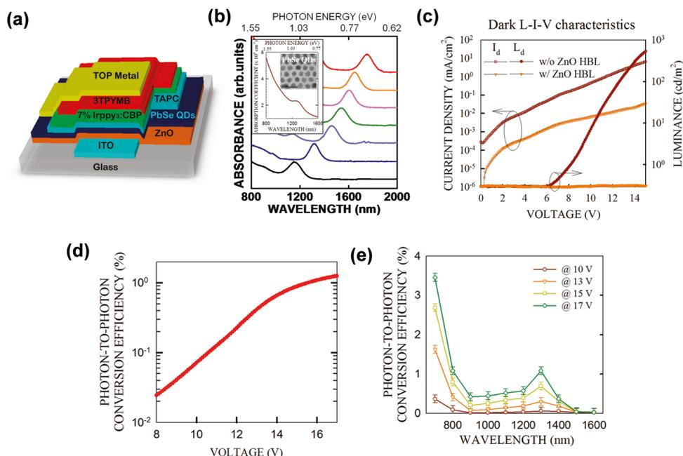
Fig. 11 (a) Schematic diagram of device structure. (b) Absorption spectra of various QDs. (c) Dark  $I$ - $V$  characteristic curves. (d) and (e) Up-conversion efficiency.<sup>37</sup> Copyright 2011, American Chemical Society.
