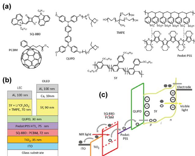
Fig. 5 (a) Organic materials of thin films. (b) Schematic diagram of structure of an all-solution organic device. (c) Organic semiconductor band diagram.<sup>75</sup> Copyright 2019, American Chemical Society.
