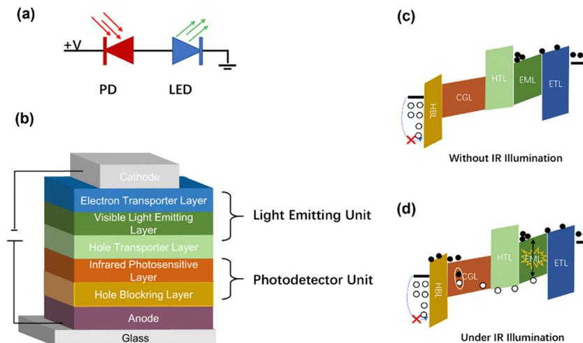
Fig. 2 (a) Schematic diagram of photodiodes. (b) Schematic diagram of the up-conversion device structure. (c) and (d) Schematic diagram of the upconverters working without IR (c) and with IR (d) illumination, respectively.
