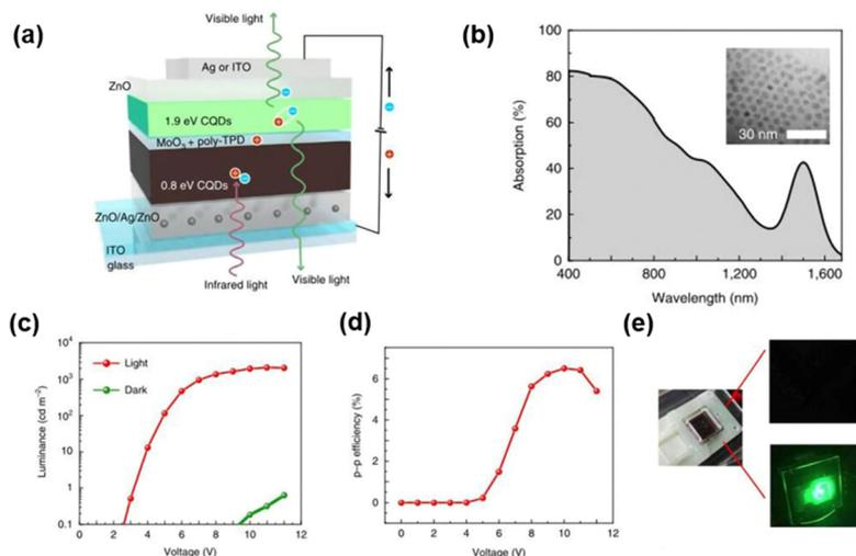
Fig. 10 (a) Schematic diagram of device structure and infrared to visible light conversion mechanism. (b) Absorption spectrum of QDs. (c)  $L$ - $V$  characteristic curves. (d) Up-conversion efficiency. (e) Schematic of on/off states.<sup>93</sup> Copyright 2020, SpringerNature.
