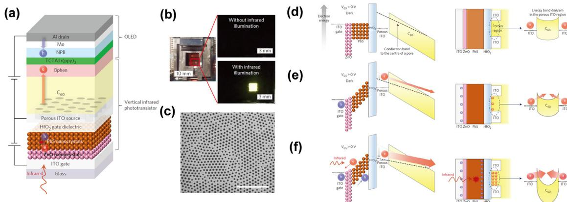
Fig. 12 (a) Schematic diagram of device structure. (b) Photos of on/off states. (c) SEM image of the porous ITO film. (d), (e) and (f) Schematic diagram of physical mechanisms.<sup>34</sup> Copyright 2016, Springer Nature.
