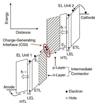
Fig. 6 Schematic of vacuum energy levels of each unit of tandem OLEDs.<sup>77</sup> Copyright 2016, WILEY-VCH Verlag GmbH.
