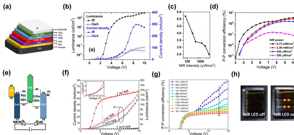
Fig. 9 (a) Schematic diagram of device structure. (b), (f) and (g)  $L$ - $V$  &  $J$ - $V$  characteristic curves. (c) Variation of turn-on voltage with NIR intensity. (d) Up-conversion efficiency. Copyright 2019, AIP Publishing. (e) Semiconductor band diagram. (h) Digital photos of on/off states.<sup>91,92</sup> Copyright 2020, The Author(s).
