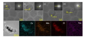
Fig. 2 (a)-(d) HR-TEM images and corresponding FFT pattern of 0%, 3%, 7%, and 13% Tm doping of CsMnCl<sub>3</sub> NCs. (e) TEM and EDS mapping images of Tm3+-CsMnCl3 NCs.
