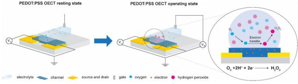
Fig. 1 A schematics of PEDOT:PSS OECT in its resting state and upon  $V_0$  operation, showing electron transfer from the polymer channel to the electrolyte and consequent generation of H2O2
