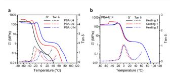
Fig. 12 DMTA curves of the PBA-UPy networks. (a) Storage modulus (G') and loss factor  $(\tan \delta)$  as a function of temperature for all polymers; (b) storage modulus (G') and tan  $\delta$  as a function of temperature for a second sample of PBA-U14 in two heating runs and one cooling run. Note that the absolute G' values are lower than expected for glassy polymers indicating that the calibration was not optimal, which will, however, not influence the relative trends
