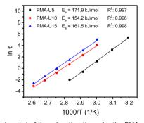
Fig. 10 Arrhenius plot of the relaxation times for the PMA-UPy networks, determined by the crossover points of G' and G'' in the frequency sweeps with apparent activation energy (Ea) obtained by linear fiting of the data.
