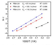
Fig. 14 Arrhenius plot of the relaxation times for the PBA-UPy networks, determined by the crossover points of G' and G'' in the frequency sweeps with apparent activation energy (Ea) obtained by linear fiting of the data.
