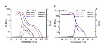
Fig. 8 DMTA curves of the PMA-UPy networks. (a) Storage modulus (G') and loss factor  $(\tan \delta)$  as a function of temperature for all polymers; (b) storage modulus (G') and tan  $\delta$  as a function of temperature for a second sample of PMA-U5 in two heating runs and one cooling run. Note that the absolute G' values are lower than expected for glassy polymers indicating that the calibration was not optimal, which will, however, not influence the
