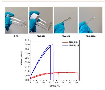
Fig. 13 Top: Physical appearance of the PBA polymer compared to PBA-UPv materials: PBA-U4 still showed viscous liquid behavior, while PBA-U9 and PBA-U14 could be compression molded and pressed into dog bones for tensile testing. Bottom: Tensile test stress-strain curves of PBA-U9 and PBA-U14.
