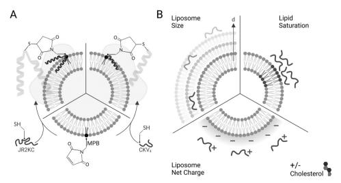
Scheme 1 (A) The thiol-containing peptides JR2KC and CKV<sub>4</sub> were conjugated to maleimide-functionalized liposomes via a Michael addition reaction, which triggered peptide folding and liposome cargo release. (B) The effect of liposome size (d), cholesterol, fraction of saturated lipids, and liposome net charge, on peptide-triggered release was explored.
