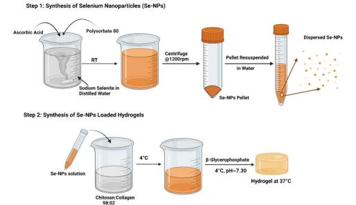
Fig. 1 Schematic diagram showing the steps followed for the synthesis of the Se-NPs and hydrogels
