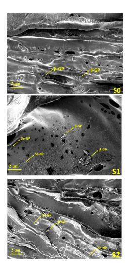
Fig. 5 Representative SEM images of Se-NPs-functionalized freeze-dried hydrogels at 50 µm magnification. Arrow indicates the presence of bright Se-NPs and  $\beta$ -GP crystals on the surface of the hydrogels.
