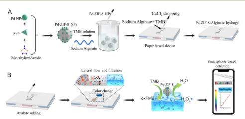
Scheme 1 Schematic illustration of PAD hydrogel-based separation-free device for H<sub>2</sub>O<sub>2</sub> detection by a smartphone.
