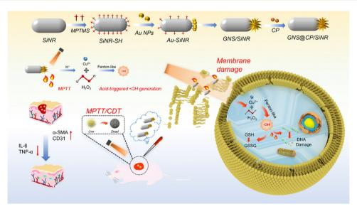
Scheme 1 Illustration of the synthetic route of the GNS@CP/SiNR Janus nanostructure, its NIR II mild photothermal effect and acid-triggered \*OH generation properties, and the synergistic MPTT/CDT antibacterial application and mechanism.
