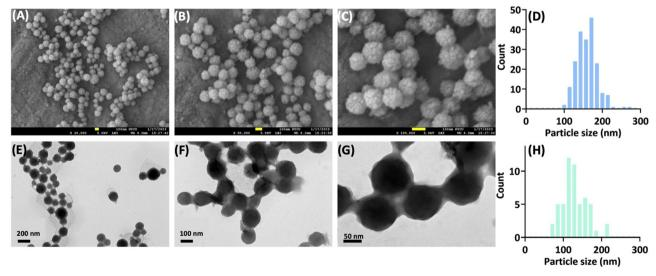
Fig. 4 Characterization of nanoparticle morphology. (A)–(C) SEM images at different magnifications (yellow bar = 100 nm). (D) Size distribution for the SEM image A. (E)-(G) TEM images at different magnifications. (H) Size distribution for the TEM image E.
