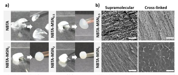
Fig. 3 Structural analysis of NBTA-MSN nanocomposites. (a) Optical images of NBTA-MSN hydrogels with various concentrations of MSNs. (b) Cryo-SEM images of NBTA-MSN<sub>0.5</sub> (scale bar: 5 μm) and NBTA-MSN<sub>1</sub> (scale bar: 5 μm before UV exposure, and 1 μm for after UV exposure) before and after MSN crosslinking upon UV exposure
