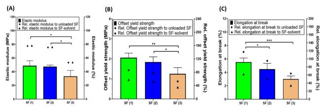
Fig. 5 Mechanical properties of the rifampicin-SFs (SmartFilms) in this study showing (A): the elastic modulus, (B): the offset yield strength and (C): the elongation at break. Unloaded SF and SF treated only with the used solvent only (without rifampicin) were used as bench controls (means + SD, n = 5).
