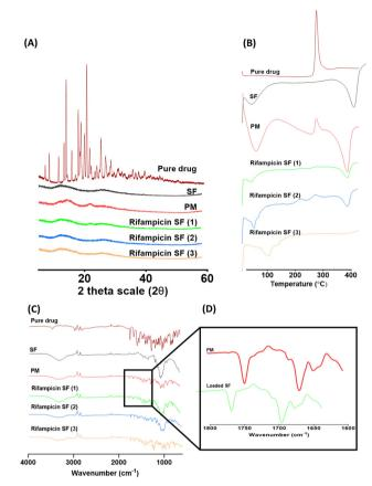
Fig. 3 Characterization of the crystallinity/amorphous state of rifampicin within the SFs (SmartFilms) and the controls (Pure drug, unloaded SF and physical mixture (PM)) in this study showing (A): X-RD diffractograms, (B): the DSC thermograms and (C): FTIR spectra. (D): FTIR spectra magnified associated with the specific groups to compare the physical mixture with the loaded representative SF.
