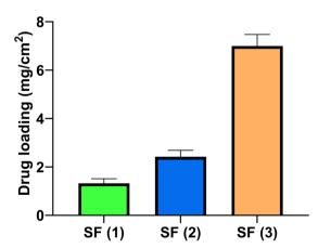
Fig. 6 The amount of rifampicin loaded within the three different SFs (SmartFilms) produced in this study expressed as mg cm<sup>-2</sup> of each SF (means + SD, n = 3). The SFs represent the SmartReservoirs (SRs) when affixed on the top of the drug free HF-MNs (hydrogel-forming MNs) in this study.
