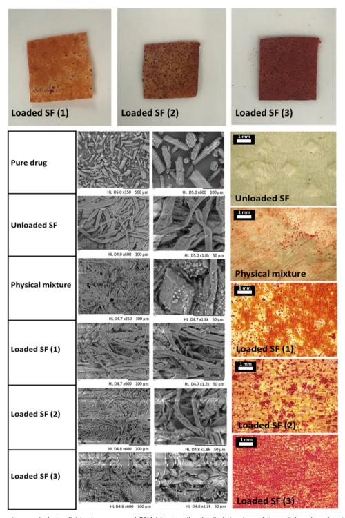
Fig. 2 Macroscopic, microscopic (using light microscope and SEM (showing the detailed structure of the cellulose-based matrix and their pores)) visualization of the obtained SFs (SmartFilms) in this study. Loaded SFs have been labelled according to drug loading, in which SF (1) represents the lowest rifampicin loading and SF (3) represents the highest rifampicin loading. Pure drug, unloaded SF and physical mixture were used as controls.
