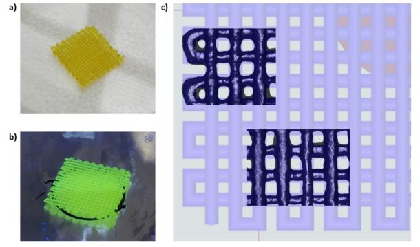
Fig. 9 (a) Photo of a 3D-printed construct based on HHP407 5%-CD 8% Cur. (b) UV curing of HHP407 5%-CD 8% Cur structures. (c) Qualitative geometrical match between the 3D-printed HHP407 5%-CD 8% Cur and the starting theoretical CAD design.
