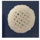
Fig. 11 (a) Photograph of HHP407 5%-CD 8%-based 25-layer cylinder construct with a 0/90° pattern taken during the 3D printing process and (b) macroscopic appearance of 3D printed 25-layer cylinder constructs with a 0/90° pattern at the end of the printing process.
