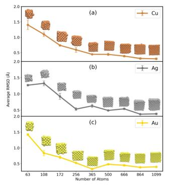
**Fig. 4** The time averaged RMSD of (a) Cu, (b) Ag, and (c) Au MNCs with respect to their sizes in the presence of a 4M IL–water mixture. The RMSD averages were performed for 100 ns time of simulation.
