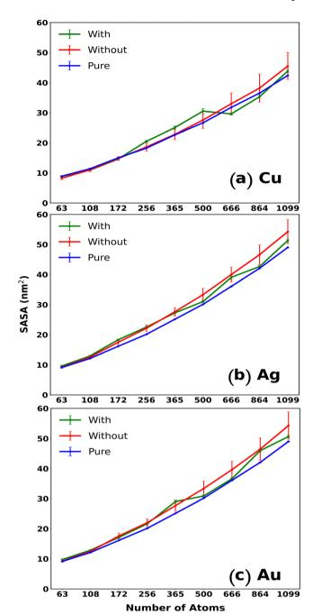
Fig. 3 The calculated SASA for different metal NCs with respect to their sizes. The blue curve denotes the SASA of the perfect cubic shaped starting structures of the respective cubic NCs. The red and the green curves denote the time averaged SASA for the respective cubic NCs over the 100 ns trajectory without and with IL respectively. It can be very well observed that the CuNCs in water and IL-water mixture exhibits considerable similarity with the starting geometries compared to Ag and Au NCs.
