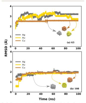
**Fig. 6** The time evolution of RMSD of Cu (brown), Ag (silver) and Au (yellow) MNCs in water for the NC size of (a) 63 and (b) 108, respectively. The comparative stability of the Cu analogues can be easily monitored herewith.
