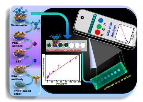
Scheme 2 Schematic representation of smartphone paper-based optical sensors for the detection of PSA cancer biomarkers.
