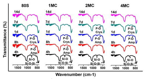
Fig. 7 FTIR spectra of MBGs between 1600 and 400 cm<sup>-1</sup> after placing them in SBF from 4 h to 14 days
