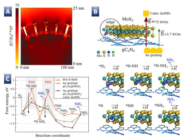
Fig. 5 (A) FDTD simulation of coupled plasmon energy distribution for the Au grating/gC<sub>3</sub>N<sub>4</sub>@MoS<sub>2</sub>/cubic AuNPs structure case; (B) DFT simulation of the NRR process on the edge of the  $gC_3N_4@MoS_2$  surface under external, plasmon-related  $\vec{E}$ ; (C) free energy profile of the NRR with and without plasmon triggering in "simple" and coupled plasmon regimes.
