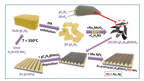
Fig. 1 Schematic representation of sample preparation
