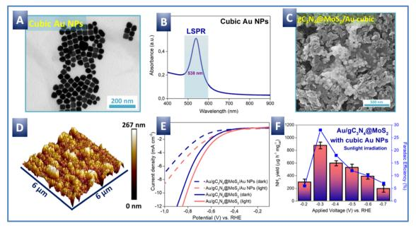
Fig. 6 (A) TEM image and (B) UV-Vis spectrum of cubic Au NPs; (C) SEM and (D) AFM images of Au/gC<sub>7</sub>N₄@MoS₂ coupled with top-deposited cubic AuNPs; (E) LSV curves measured on the Au/gC<sub>3</sub>N<sub>4</sub>@MoS<sub>2</sub> and Au/gC<sub>3</sub>N<sub>4</sub>@MoS<sub>2</sub>/AuNPs surface with and without light illumination; (F) NH<sub>3</sub> yield and faradaic efficiency obtained on the Au/qC<sub>3</sub>N₄@MoS₂/AuNPs surface in the photoelectrochemical regime.
