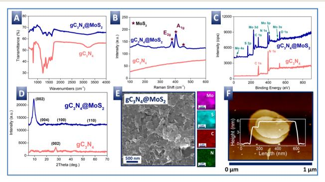
Fig. 2  $gC_3N_4@MoS_2$  characterization: (A)–(C) FT-IR, Raman, and XPS spectra; (D) XRD patterns; (E) SEM-EDX image with elemental mapping and (F) AFM images of  $gC_3N_4@MoS_2$  flakes and the single flake profile.
