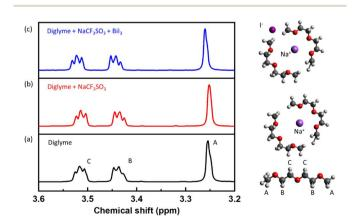
Fig. 2  $^{1}$ H NMR spectra of (a) pure diglyme solvent, (b) diglyme with sodium salt (NaCF<sub>3</sub>SO<sub>3</sub>), and (c) diglyme with sodium salt (NaCF<sub>3</sub>SO<sub>3</sub>) and additives (Bil<sub>3</sub>). Deuterated DMSO is used as the reference solvent for all three testing studies.
