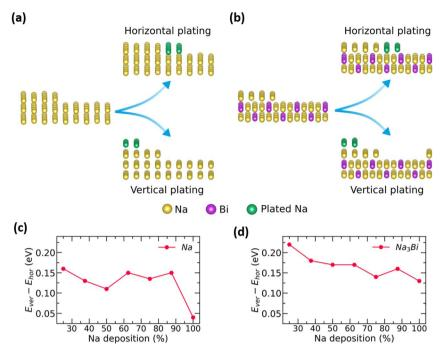
Fig. 5 Schematic representation illustrating the horizontal and vertical plating mechanisms of Na on (a) bulk Na-metal and (b)  $Na_3Bi$  surfaces. The graphs below show the variation in the energy difference between vertical and horizontal plating in response to varying Na deposition concentrations for (c) bulk Na-metal and (d)  $Na_3Bi$  surfaces.
