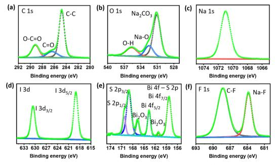
Fig. 6 High-resolution XPS spectra of Na metal cycled in 100 mM Bil<sub>3</sub>-added electrolyte for 20 cycles. (a) C 1s, (b) O 1s, (c) Na 1s, (d) I 3d, (e) Bi 4f– S 2p and (f) F 1s spectra.
