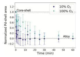
Fig. 5 In situ STEM visualizing the alloying of Au-Pd core—shell NPs in  $O_2$  at 375 °C. The plot shows the normalized Pd-shell area as a function of time for a 10%  $O_2$  in Ar (dark blue) and 100%  $O_2$  (light blue) gas atmosphere. The error bars represent the standard deviation of the Pd shell related area across measurements in multiple nanoparticles.
