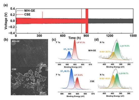
Fig. 6 Li compatibility of the M/H-GE: (a) long-term cycling of the Li|M/H-GE||Li cell and Li||CSE||Li cell at 0.1 mA cm<sup>-2</sup>, and 0.1 mA h cm<sup>-2</sup> Li plated and stripped per cycle. (b) SEM image of the deposited lithium surface after 25 cycles using different electrolytes. XPS (c) F 1s and (d) N 1s spectra of the cycled Li electrode taken from the Li||M/H-GE||Li cell and Li||CSE||Li cell.
