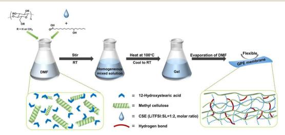
Fig. 1 Schematic illustration of the preparation of the M/H-GE membrane using MC, 12-HOA, and CSE (LiTFSI: SL = 1:2).
