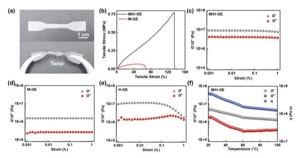
Fig. 3 Mechanical properties of GEs: (a) digital photographs of the twisted M/H-GE membrane. (b) Tensile stress-strain curves of the M-GE and M/H-GE membranes. Strain-dependent storage modulus (G') and loss modulus (G'') curve of (c) M/H-GE, (d) M-GE, and (e) H-GE membranes. (f) Temperature-dependent rheological curves of the M/H-GE membrane (angular frequency = 10 rad s<sup>-1</sup>, strain = 1%).
