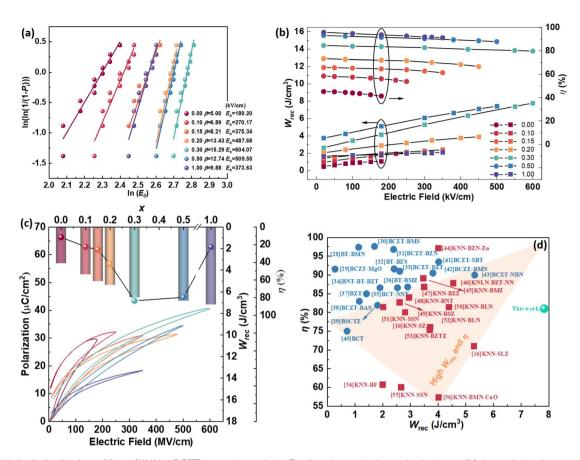
Fig. 3 (a) Weibull distribution of (1 - x)KNN - xBCZT ceramics and the  $E_b$  of each one is shown in the inset; (b) the variation between both  $W_{rec}$ and  $\eta$  and applied electric field; (c) the P-E loops at  $E_b$  of all the ceramics are summarized at the bottom, and the  $W_{rec}$  and  $\eta$  of each ceramic are plotted on the top; (d) the comparison between the 0.7KNN-0.3BCZT ceramic in this work and some typical BCZT-based and KNN-based ceramics.16,28-56
