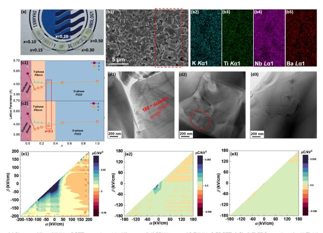
Fig. 1 (a) Picture of (1 - x)KNN - xBCZT ceramics with different x; (b1) SEM image of 0.7KNN - 0.3BCZT; (b2) - (b5) EDS mappings for K, Ti, Nb, and Ba of the area circled by the red dashed rectangle in (b1); (c1) and (c2) the variation between the lattice parameter and x; (d1)–(d3) TEM images of (1-x)KNN-xBCZT ceramics with x = 0.1. 0.3, and 0.5; (e1)-(e3) the FORC distribution of (1-x)KNN-xBCZT ceramics with x = 0.1. 0.3, and 0.5.
