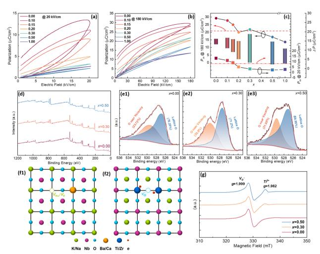
Fig. 4 The unipolar P-E loops of (1-x)KNN-xBCZT ceramics under (a) 20 kV cm $^{-1}$ ; (b) 180 kV cm $^{-1}$ ; (c) the variation between the  $P_{\rm m}$  in (a) and (b) and x with the difference between them; (d) the XPS spectrum from 0–1200 eV; (e1)–(e3) the enlarged XPS spectrum from 524–536 eV; (g) the EPR spectrum of (1-x)KNN-xBCZT ceramics with x=0.00, 0.30, and 0.50; (f1) and (f2) sketch of the A-O plane and B-O plane of the lattice of (1-x)KNN-xBCZT ceramics to explain eqn (1)–(9).
