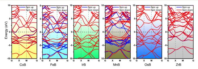
Fig. 3 Band structures of six dynamically stable anti-MXene boride monolayers (CoB, FeB, IrB, MnB, OsB, and ZrB) depicting spin-resolved electronic states. The Fermi level is delineated by the dashed horizontal line at zero energy, with spin-up and spin-down states represented by red and blue lines, respectively. The presence of bands crossing the Fermi level indicates metallic behavior in these materials.
