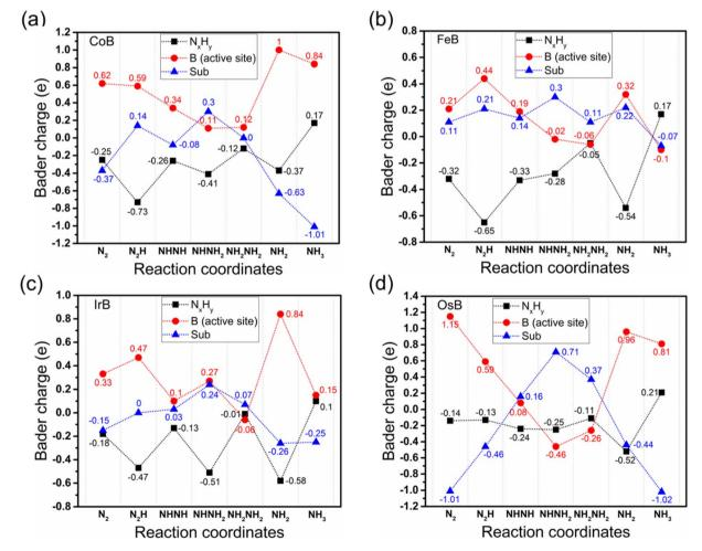
Fig. 7 Bader charge analysis along the reaction coordinates for the alternating NRR pathway on (a) CoB, (b) FeB, (c) IrB and (d) OsB. The plots trace the charge variations for  $NH_x$  intermediates (black dotted lines), the active boron site (red solid lines), and the substrate (blue dashed lines), elucidating the electron transfer dynamics during the catalytic process.
