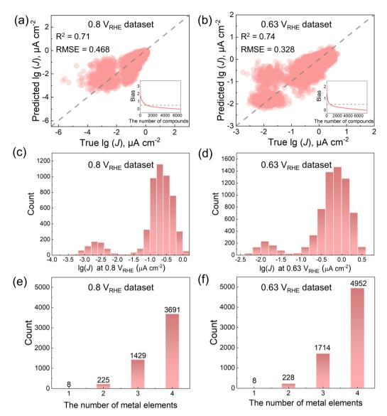
Fig. 3 (a and b) Performance of the initial ANN model based on the 10-fold cross validation in the (a)  $0.8\,V_{RHE}$  and (b)  $0.63\,V_{RHE}$  datasets. (c and d) Distribution of current densities after cleaning the noisy data in the (c)  $0.8 \, V_{RHE}$  and (d)  $0.63 \, V_{RHE}$  datasets. (e and f) Statistics of the materials with various number of elements in the (e)  $0.8 V_{RHE}$  and (f)  $0.63 V_{RHE}$  datasets.
