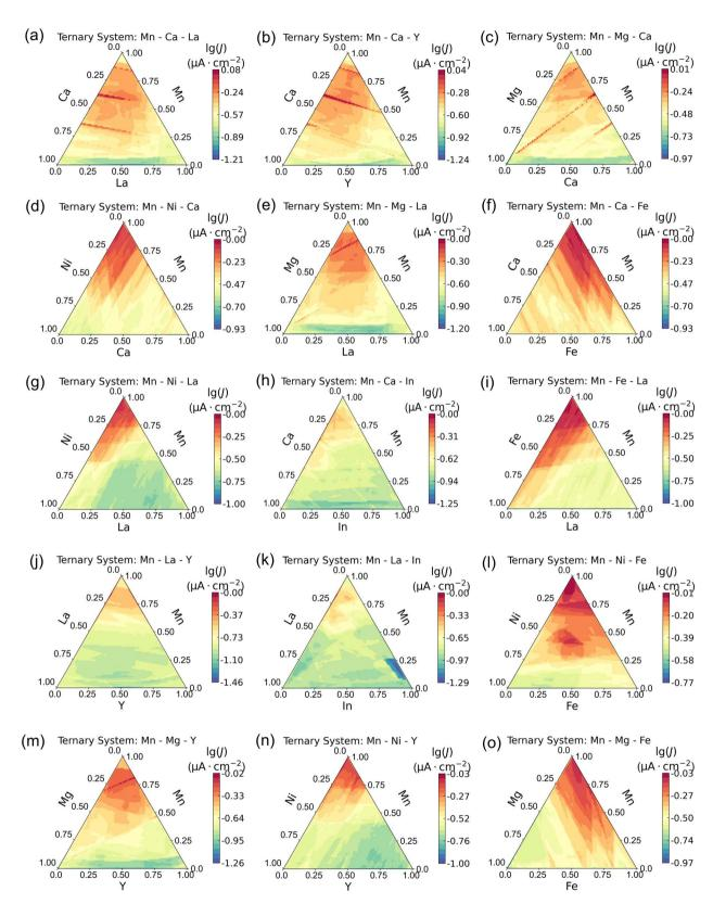
Fig. 6 Predictive current density values at  $0.8 \text{ V}_{\text{RHE}}$  for the fifteen ternary systems based on the trained XGBoost model. (a–o) Ternary systems of (a) Mn–Ca–La, (b) Mn–Ca–Y, (c) Mn–Mg–Ca, (d) Mn–Ni–Ca, (e) Mn–Mg–La, (f) Mn–Ca–Fe, (g) Mn–Ni–La, (h) Mn–Ca–In, (i) Mn–Fe–La, (j) Mn–La–Y, (k) Mn–La–In, (l) Mn–Ni–Fe, (m) Mg–Mg–Y, (n) Mn–Ni–Y, and (o) Mn–Mg–Fe.
