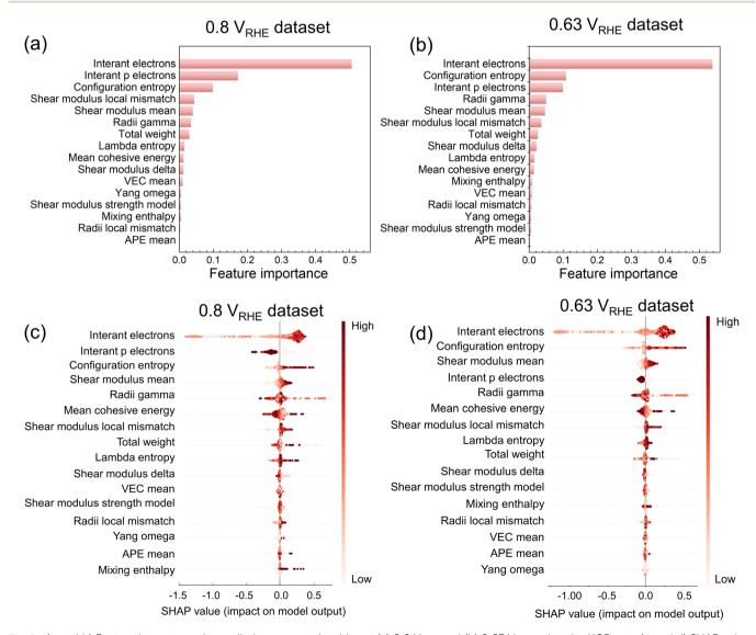
Fig. 5 (a and b) Feature importance in predicting current densities at (a)  $0.8 \text{ V}_{\text{RHE}}$  and (b)  $0.63 \text{ V}_{\text{RHE}}$  using the XGBoost. (c and d) SHAP values derived from the XGBoost model in the (c)  $0.8 V_{RHE}$  and (d)  $0.63 V_{RHE}$  datasets.
