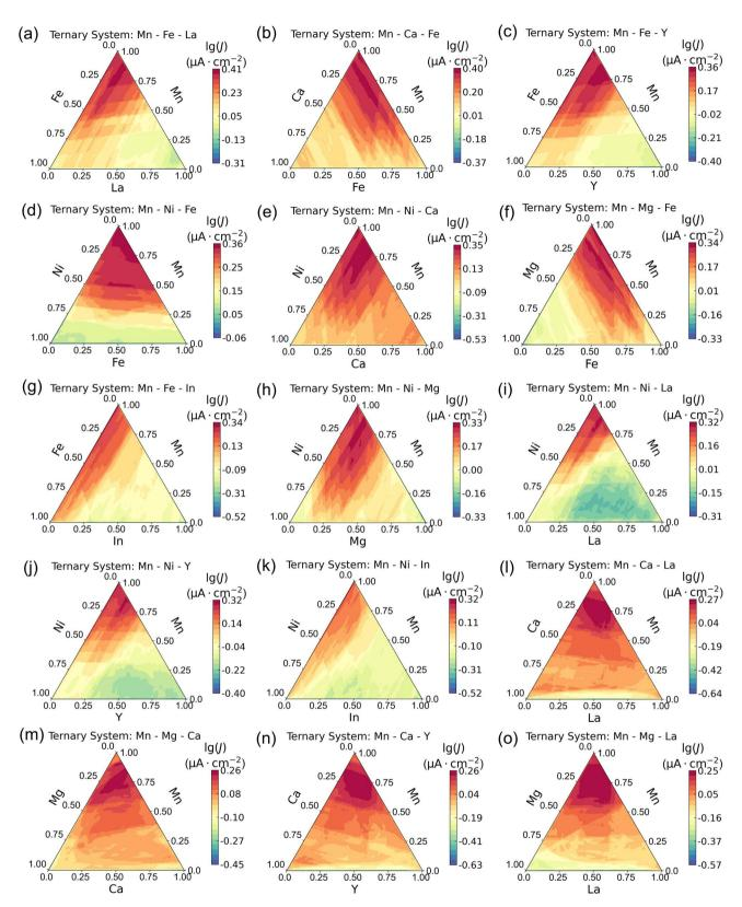
Fig. 7 Predictive current density values at  $0.63 \, V_{RHE}$  for the fifteen ternary systems based on the trained XGBoost model. (a–o) Ternary systems of (a) Mn-Fe-La, (b) Mn-Ca-Fe, (c) Mn-Fe-Y, (d) Mn-Ni-Fe, (e) Mn-Ni-Ca, (f) Mn-Mg-Fe, (g) Mn-Fe-In, (h) Mn-Ni-Mg, (i) Mn-Ni-La, (j) Mn-Ni-Y, (k) Mn-Ni-In, (l) Mn-Ca-La, (m) Mg-Mg-Ca, (n) Mn-Ca-Y, and (o) Mn-Mg-La.
