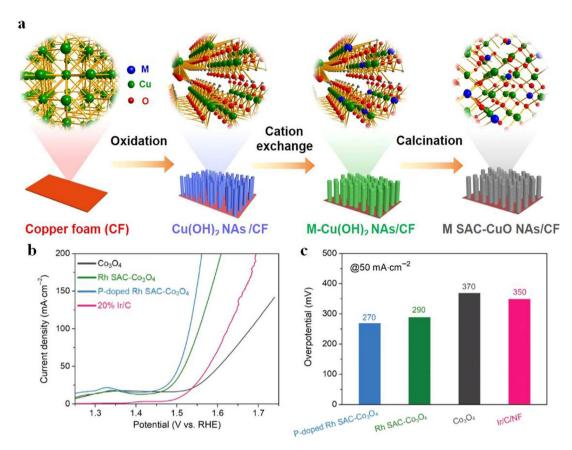
Fig. 4 (a) Schematic representation and corresponding atomic structure of the products. Reproduced with permission.<sup>52</sup> Copyright 2020 American Chemical Society (b) OER polarization curves and (c) overpotentials at 10 and 50 mA cm<sup>-2</sup>. Reproduced with permission.<sup>53</sup> Copyright 2022, Springer Nature.
