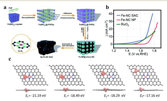
Fig. 8 (a) Self-template synthesis process of the Fe-NC SAC. (b) The Fe-NC SAC, Fe-NC NP and Pt/C OER polarization curves of the OER at 1600 rpm; Reproduced with permission.<sup>65</sup> Copyright 2020, Royal Society of Chemistry; (c) the formation energy of different configurations of Fe clusters and Fe-N4 sites. Reproduced with permission.<sup>67</sup> Copyright 2022, Wiley-VCH Verla.
