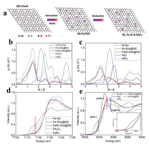
Fig. 9 (a) Synthesis process of the Ni-O-G SACs. Reproduced with permission. 72 Copyright 2019, Elsevier. (b) Fe K-edge FT-EXAFS spectra. (c) Ni K-edge FT-EXAFS spectra. (d and e) XANES at the Fe K-edge and Ni K-edge. Reproduced with permission.73 Copyright 2022, Elsevier.
