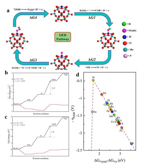
Fig. 5 (a) Schematic of the  $4e^-$  OER pathway of the 4H site via the  $M_1/PMA$  cluster, reproduced with permission. Chemical Society. (b) Free energy diagrams of basic steps of the Pd@Sb monolayer and (c) Pd@Sb monolayer at different potentials. (d) The volcano curve between negative OER overpotential and  $\Delta G_{OOH^*} - \Delta G_{O^*}$  for TM@Sb monolayers. Reproduced with permission. Copyright 2021, Royal Society of Chemistry.
