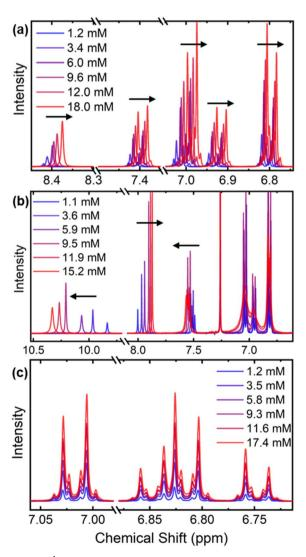
Fig. 3 Partial <sup>1</sup>H-NMR spectra of (a) compound 1 and (b) compound 3 at different concentrations, showing shifts in their amide and aromatic proton resonances, and (c) compound 2, showing no shifts across the concentration range.
