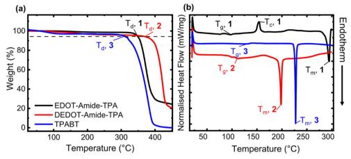
Fig. 2 Stacked (a) TGA and (b) DSC curves for our three amide HTMs. Thermograms were recorded for pristine HTMs, at a rate of 5 °C min<sup>-1</sup> under nitrogen.
