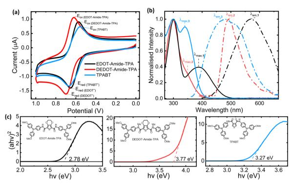
Fig. 1 (a) Cyclic voltammograms referenced to the Fc/Fc<sup>+</sup> redox couple (CH<sub>2</sub>Cl<sub>2</sub>,  $1 \times 10^{-4}$  M), (b) solution UV-visible absorption (solid lines) and emission spectra (dashed lines) of the three amide-based HTMs, and (c) Tauc plots and corresponding optical bandgaps  $E_{\rm q}$ .
