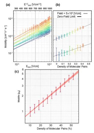
Fig. 10 (a) Mobility against field at different pair densities, (b) mobility against pair density at a field strength of  $5 \times 10^5 \, \mathrm{V \ cm^{-1}}$  and at zero field, (c) normalised mobility against pair density.
