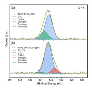
Fig. 4 XPS data for O 1s core level spectra of (a) the pristine TAPB-DHTA-COF and (b) TAPB-DHTA-COF@Fe, including a line shape analysis and deconvolution of the peaks.
