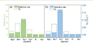
Fig. 3 Adsorption selectivity test of (a) TAPB-PDA-COF, and (b) TAPB-DHTA-COF in the presence of other cations: Ca<sup>2+</sup>, Mg<sup>2+</sup>, Mn<sup>2+</sup>, Na<sup>+</sup>,  $Fe^{2+}$ , and,  $K^+$ .  $C_{Ca} = 1.715$  ppm,  $C_{Mg} = 0.982$  ppm,  $C_{Mn} = 1.095$  ppm,  $C_{\mathrm{Na}}=0.376$  ppm,  $C_{\mathrm{Fe}}=0.177$  ppm, and  $C_{\mathrm{K}}=0.283$  ppb.
