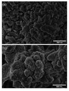
Fig. 1 SEM images of (a) TAPB-PDA-COF and (b) TAPB-DTHA-COF.
