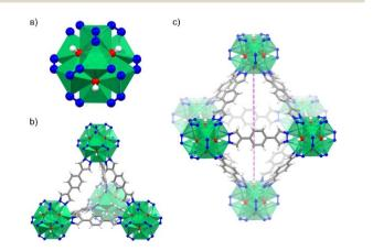
Fig. 1 (a) Structure of the octanuclear Ni(II) cluster in  $[Ni_8(OH)_4(H_2-O)_2(BDP)_6]$ . (b) View of the tetrahedral, and (c) octahedral cages found in the crystal structure of NiBDP MOF. Color code: Ni (green); N (blue); O (red); C (grey) and H (white).
