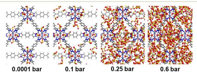
Fig. 5 GCMC simulated adsorption sequence of SO<sub>2</sub> in NiBDP-0H<sub>2</sub>O at 298 K, and at different pressures. SO<sub>2</sub> atom color codes: red (O), yellow (S). MOF atom color codes: red (O), gray (C), blue (N), white (H), purple (Ni).
