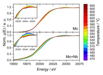
Fig. 9 Normalized XANES at the Mo K-edge recorded *in situ* of 6Mo/HZSM-5 (top) and 6Mo1Nb/HZSM-5 (bottom) during continuous heating. Curves depict the normalized sum of 10 measurements (60 s) in the range of  $T\pm5$  °C. Insets show zoom-ins on the edge features. Reaction conditions: 50 mL min<sup>-1</sup> 20% CH<sub>4</sub>/N<sub>2</sub>, 1 atm, heating rate 10 °C min<sup>-1</sup>, heating from RT to 600 °C.
