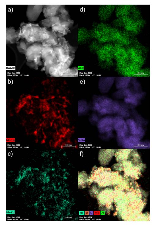
Fig. 5 STEM micrograph (a) and the corresponding EDS maps ((b) Mo L $\alpha$ ; (c) Nb K $\alpha$ ; (d) Al K; (e) Si K $\alpha$ ; (f) overlay of O, Si, Al, Mo and Nb) of the fresh 6Mo1Nb/HZSM-5 catalyst.
