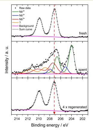
Fig. 7 Intensity-normalized XP spectra for the Nb 3d level of the 6Mo1Nb/HZSM-5 catalyst before the reaction (bottom), after the reaction with methane at 700 °C for 360 min (middle) and after four reaction/regeneration cycles. Reaction conditions: 700 °C, 300 mg catalyst, 90% CH $_4$  + 10% N $_2$ , 3200 SCC  $g_{cat}^{-1}\ h^{-1}$ , 1 atm, 6 h. Regeneration: 450 °C, air, 1100 SCC  $g_{cat}^{-1}\ h^{-1}$ , 1 atm, 45 min.
