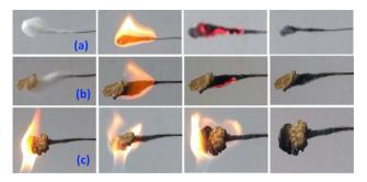
Fig. 5 Photograph of the flame-retardant test of (a) cotton without the polymer and (b) a small film of 2 wrapped over cotton, and (c) 2 direct ignitions for 2 min.
