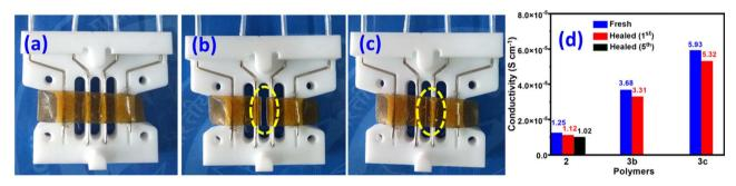
Fig. 6 Images of (a) fresh, (b) cut and (c) healed polymer membranes of 2 used for ionic conductivity measurement. (d) Ionic conductivity of fresh and healed polymers of 2, 3b, and 3c.
