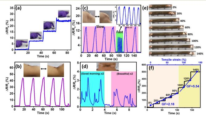
Fig. 7 Real-time monitoring of the PVIM-PPA-Ca (3c) ionogel-based wearable strain sensor for various human activities. Signals of the relative resistance change ( $\Delta R/R_0$ ) of 3c as a function of (a) finger bending at various angles, (b) arm bending, (c) knee bending, and (d) speaking different words; (e) photograph of 3c at various applied strains; (f) corresponding relative resistance ( $\Delta R/R_0$ ) and gauge factors.
