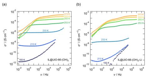
Fig. 6 (a) Conductivity isotherms of the pure activated UiO-66-(OH)<sub>2</sub> MOF with 30 wt% EMIM-FSI ionic liquid. (b) Conductivity isotherms of the UiO-66-(OH)<sub>2</sub> MOF grafted with lithium 3-methyl-3-pentoxide and containing 30 wt% EMIM-FSI ionic liquid. In this case, there is little difference between the pristine and the grafted sample at room temperature, although a decrease in conductivity can be seen for the grafted sample.
