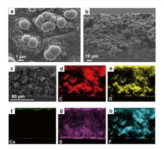
Fig. 4 (a) Surface and (b and c) cross-section morphology of PE-Co after cycling and elemental mapping of (d) C, (e) O, (f) Co, (g) S and (h)
