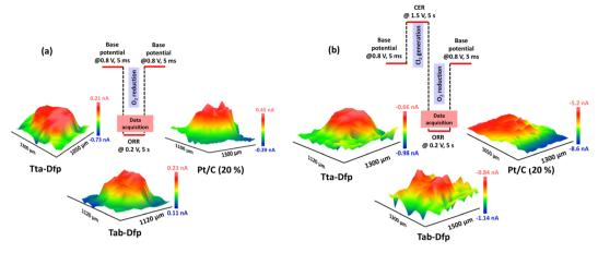
Fig. 5 Potential pulse profile for (a) only the ORR and (b) Cl<sub>2</sub> generation followed by the ORR at the Pt-tip and the corresponding 3D RC-SECM images of Tta-Dfp, Tab-Dfp and Pt/C (20%) measured in 400 mM HCl.
