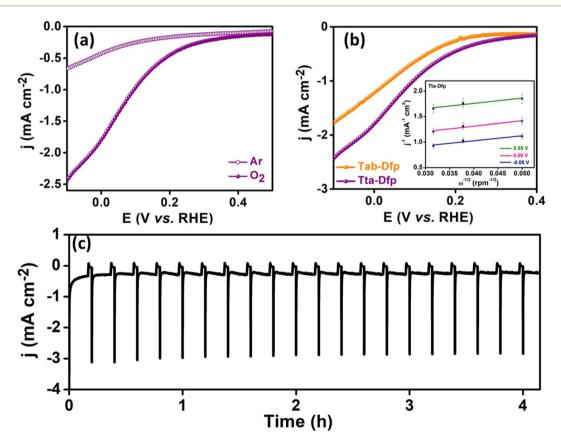
Fig. 3 (a) LSV curves for Tta-Dfp in Ar and O<sub>2</sub> saturated 0.4 M HCl electrolyte for the ORR at a rotation rate of 400 rpm, (b) LSV curves of Tta-Dfp and Tab-Dfp in O2 saturated 0.4 M HCl electrolyte (inset displaying the K-L plot for Tta-Dfp) at a rotation rate of 400 rpm, and (c) chronoamperometric analysis performed for 10 minutes of operation at 0.0 V and 2 minutes of shutdown (i.e. system off) for the Tta-Dfp catalyst.
