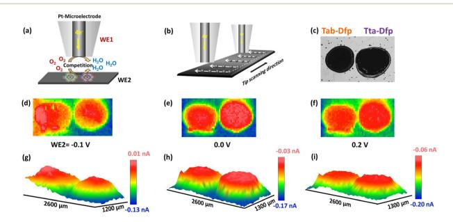
Fig. 4 (a) Schematic representation of RC-SECM mode (WE1: Pt microelectrode and WE2: catalyst coated GC plate), (b) SECM array scan, (c) microscopic images of **Tta-Dfp** and **Tab-Dfp** over the GC plate, 2D RC-SECM images of **Tta-Dfp** and **Tab-Dfp** spots measured in 400 mM HCl with different applied sample potentials: (d) -0.1 V, (e) 0.0 V, (f) 0.2 V and (g-i) their corresponding 3D images respectively. The tip (Pt-microelectrode) was polarized at 0.2 V.
