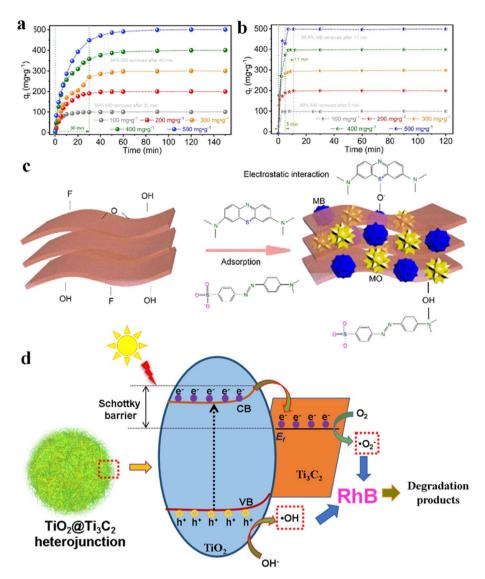
Fig. 23 (a) Adsorption of methyl orange on Nb<sub>2</sub>CT<sub>x</sub> and (b) adsorption of methylene blue at various contact times. (c) Dye adsorption via electrostatic interactions, reproduced from ref. 363 with permission from American Chemical Society, copyright 2021. (d) Photocatalytic degradation of RhB via TiO<sub>2</sub>@Ti<sub>3</sub>C<sub>2</sub>, reproduced from ref. 364 with permission from Elsevier, copyright 2021.
