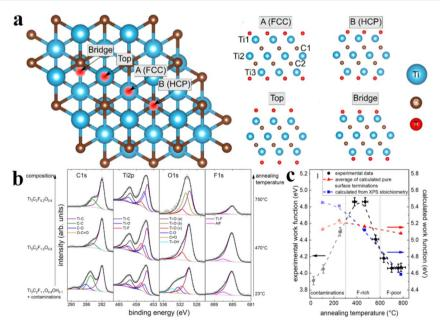
Fig. 9 (a) Adsorption sites on  $Ti_3C_2T_x$  according to DFT calculations. The FCC adsorption site is located on top of a Ti atom in the third atomic layer. HCP was exhibited on top of a C atom in the second atomic layer. (b) XPS core-level spectra of  $Ti_3C_2T_x$ . (c) Work functions of different surface terminations calculated by DFT, reproduced from ref. 152 with permission from American Chemical Society, copyright 2019.
