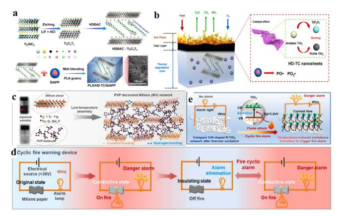
Fig. 25 (a) Synthetic scheme for HDBAC- $T_{i3}C_2T_x$  and PLA/HD-TC/SiAPP. (b) Flame-retardant mechanism, reproduced from ref. 373 with permission from Elsevier, copyright 2022. (c) Low-temperature assembly for PVP-decorated MXene paper. (d) MXene paper-based fire-detecting sensing device (schematic). (e) Resistance transition mechanism of a C/N-doped  $T_{i0}$  network, reproduced from ref. 374 with permission from Elsevier, copyright 2022.
