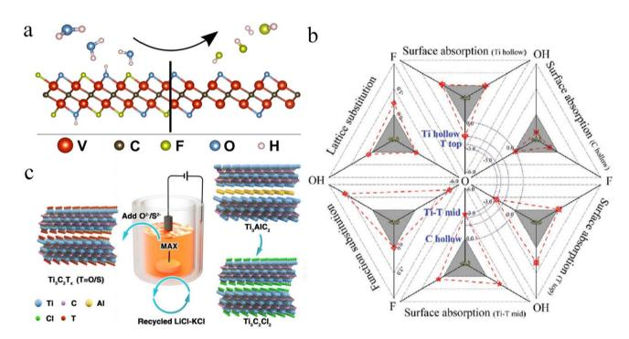
Fig. 8 (a) Removal of fluoride terminations by gas hydrolyzation, reproduced from ref. 147 with permission from American Chemical Society, copyright 2022. (b) Simulation with nitrogen dopants in  $Ti_3C_2$ , reproduced from ref. 149 with permission from Wiley, copyright 2020. (c) MXene synthesis by molten salt etching, reproduced from ref. 151 with permission from Wiley, copyright 2021.
