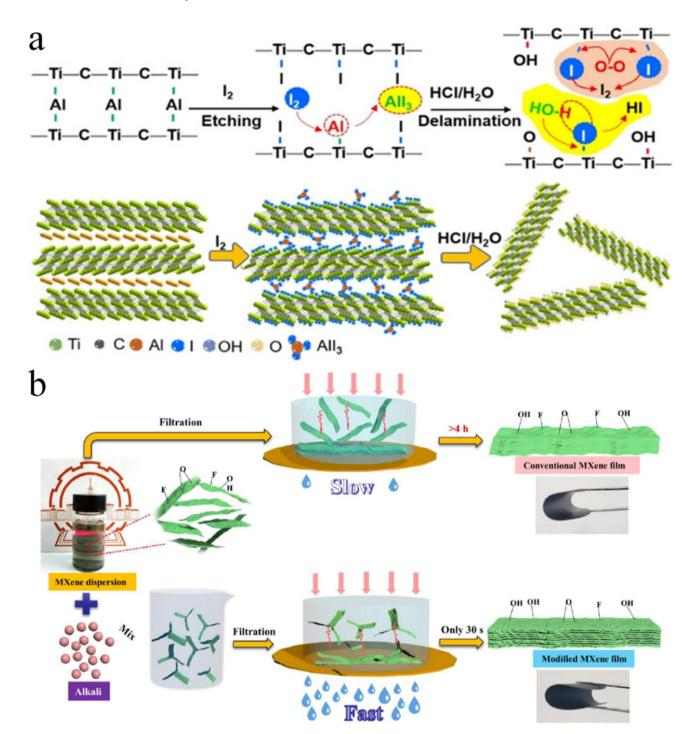
Fig. 6 (a) lodine-assisted etching and delamination of  $Ti_3AlC_2$ , reproduced from ref. 110 with permission from Wiley, copyright 2021. (b) Schematic illustration of synthesis, reproduced from ref. 111 with permission from Engineered Science, copyright 2021.
