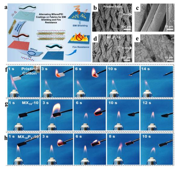
Fig. 24 (a) Assembly of a MXene/PEI-coated fabric. (b and c) SEM images of pristine cotton fabric. (d and e) SEM images of  $MX_{10}P_1-10$ . (f-h) Investigation of the fireproof properties of  $MX_{10}$ -10 and  $MX_{10}P_1$ -10 fabrics, reproduced from ref. 370 with permission from American Chemical Society, copyright 2021.
