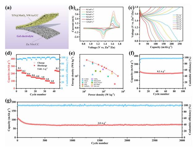
Fig. 6 Electrochemical performances of the as-assembled flexible ZIBs. (a) Schematic illustration. (b) CV curves at different scan rates. (c) GCD curves at various current densities. (d) Rate performance at various current densities from 0.1 to 4.0 A g<sup>-1</sup>. (e) Ragone plot of TiN@MnO<sub>2</sub> NWAs/ CC//Zn NSs/CC battery compared with previously reported flexible ZIBs. Cycling performance at 0.2 A  $q^{-1}$  (f) and 2.0 A  $q^{-1}$  (g).
