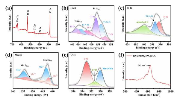
$Fig. \ 3 \quad \text{(a) Full XPS survey spectrum of TiN@MnO}_2 \ NWAs/CC \ and \ high-resolution \ Ti \ 2p \ (b), \ N \ 1s \ (c), \ Mn \ 2p \ (d), \ and \ O \ 1s \ (e) \ XPS \ spectra. \ (f) \ Raman \ (f$ spectrum of TiN@MnO2 NWAs/CC.
