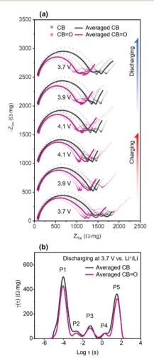
Fig. 4 (a) Nyquist plots of pristine CB and CB=O (72 h) at 3.7, 3.9, and 4.1 V vs. Li<sup>+</sup>/Li during charging and discharging. The dotted lines denote measurement of individual cells and solid lines are averages. (b) Distribution of relaxation times (DRT) of averaged pristine CB and CB= O (72 h) at 3.7 V vs. Li<sup>+</sup>/Li discharging
